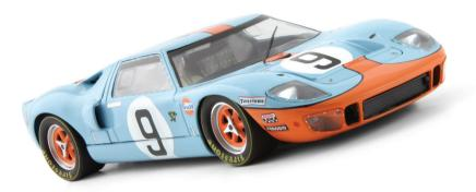
The car had a steel and aluminum semi-monocoque chassis, a body made of fiberglass and a V8 engine, originally 4.7 liter, than enlarged to a 4.9 liter.
